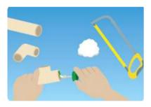
d) Push the pipe firmly into the fitting and provide a 1/4 turn. Press them for approximately 30 seconds. Remove excess cement with a clean cloth and let it dry.
