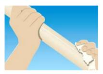
b) Cut the pipes squarely using recommended cutters or a hacksaw. Remove debris with the aid of a blade, making sure that the surface is smooth. The surface must not be sanded.
