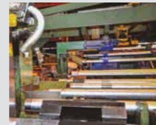
Extraction system of tubes from molten bath of zinc during hot dip galvanising of tubes
