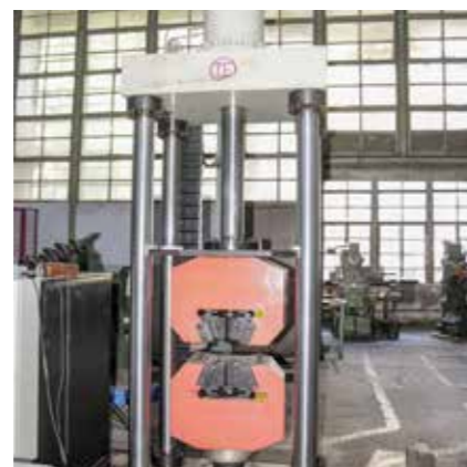
Tensile Test in progress
