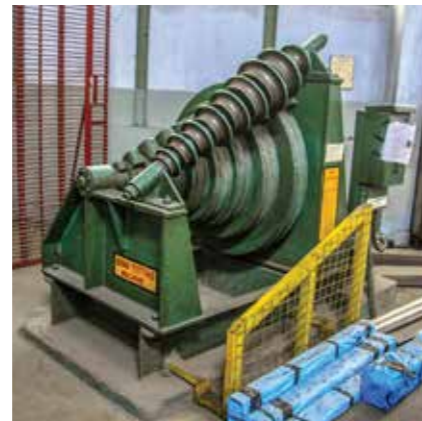
Bend testing machine used for checking weld quality and zinc coating
